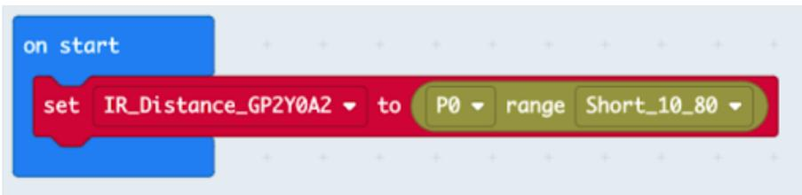
Now let's experiment with IR distance sensing by displaying the distance from your sensor to different obstacles within 10-80cm in front of it. To do this, grab the “show number” block as shown here: →
