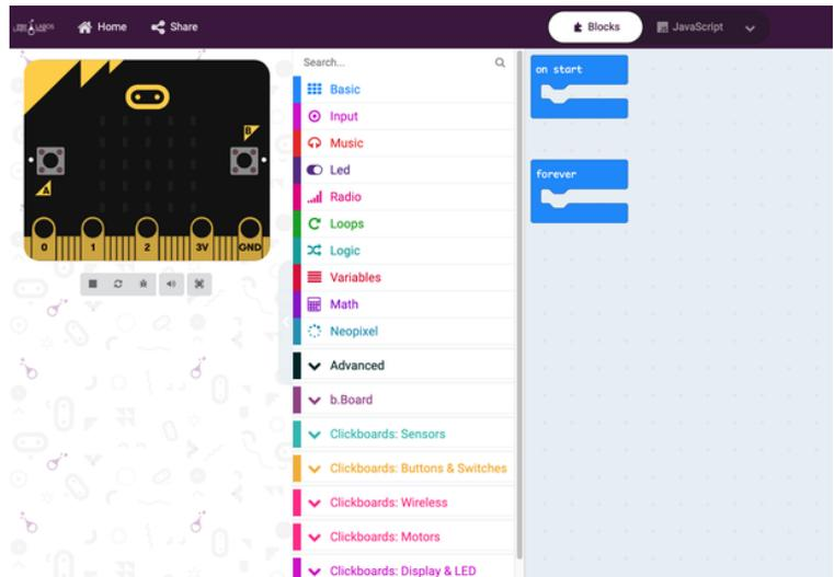
Let’s experiment with vibration detection by displaying the acceleration of the b.Board on the micro:bit LED screen. To do that, grab the “show number” block as shown here:
