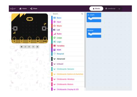
If you're using a Click Board<sup>™</sup> you'll see there is a section of dropdown toolboxes where you can find the exact Click board<sup>™</sup> you're using. In this case, we are using the Weather click which "senses" weather, so you can find it under the ClickBoards: Sensors toolbox category here:
